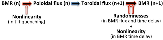
Figure 12. Schematic diagram of our BL dynamo model with nonlinearities and randomness involved in it (see text for discussion). Here n refers to the cycle number.
